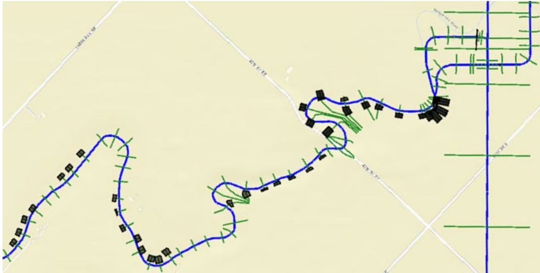
Figure 21. HEC-RAS geometry representation of the Sheyenne River Proposed Alternative with benching represented by black rectangles
