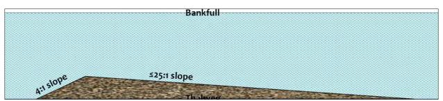
Figure 6-10: Generic Riffle Longitudinal Profile View Detail (Minnesota DNR)
