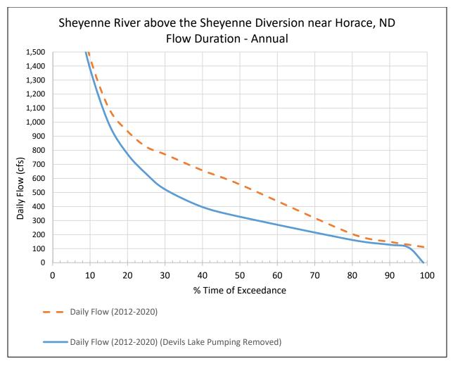
Figure 12. Flow duration curve comparison after removing Devils Lake pumping flows - annual
