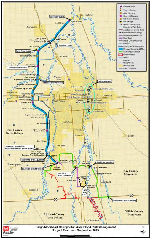
Figure 2 – Diversion Channel and Dam Alignments and Other Project Features
