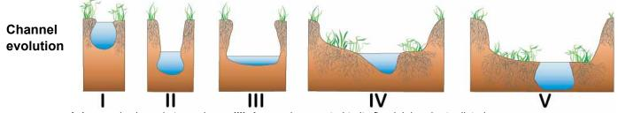
I. A properly shaped stream in equilibrium and connected to its floodplain prior to disturbance.
