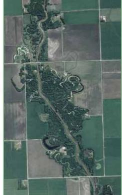
Land use change and channelization: The floodplain and stream corridor are impinged by agricultural fields. The meanders are disconnected after straightening by channelization.
