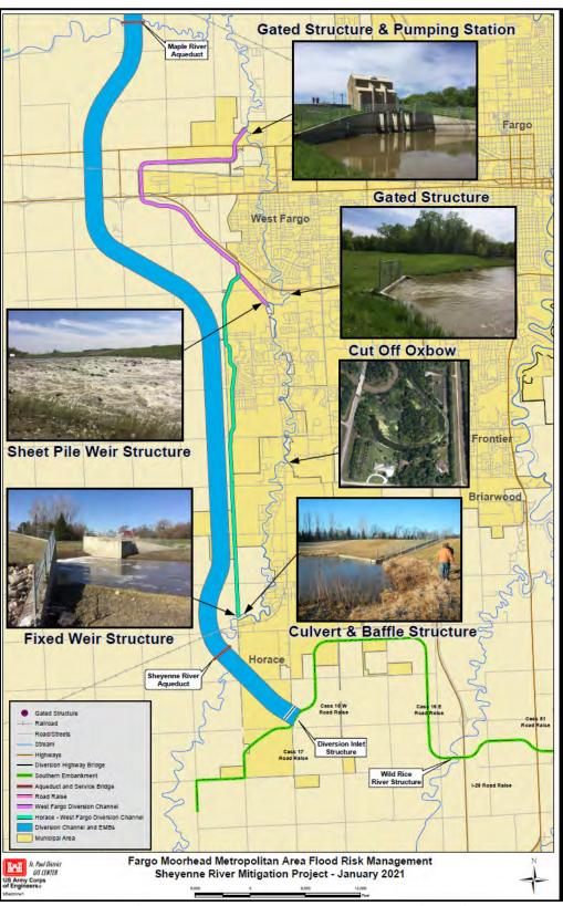
Figure 1. Overview of the Sheyenne River Flood Control Project (SRFCP) and associated features of the Sheyenne mitigation project.
