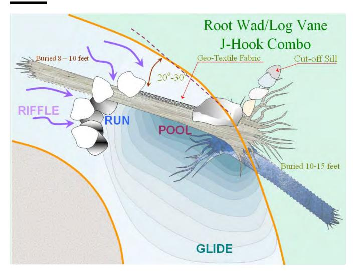
Figure 11–35 Log vane/J-hook combo with rootwad structure
