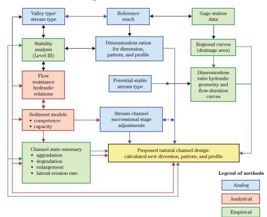
Figure 11–17 Flowchart for determining sediment supply and stability consequences for river assessment
