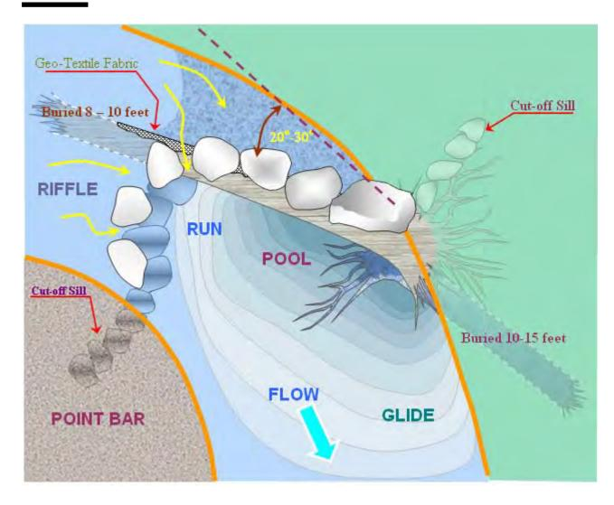
Figure 11–37Native boulder J-hook with cut-off sill,<br/>East Fork Piedra River, CO
