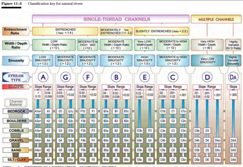
KEY to the ROSCEN CLASSIFICATION of NATURAL RIVERS. As a function of the "continuum of physical variables" within stream reaches, values of **Entrenchment** and **Sinuosity** ratios can vary by +/- 0.2 units; while values for **Width / Depth** ratios can vary by +/- 2.0 units.
