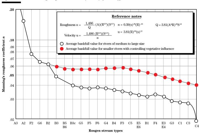
Figure 11–8 Bankfull stage roughness coefficients (*n* values) by stream type for 140 streams in the United States and New Zealand
