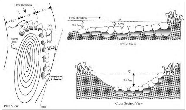
Figure 6-6: Generic J-Hook Vane Plan, Profile, and Cross-Sectional View Detail
