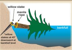
\* Tree revetments work best in small to medium streams with high sand or gravel loads because sediment deposition is important to the long-range goal of rebuilding and protecting the bank.
