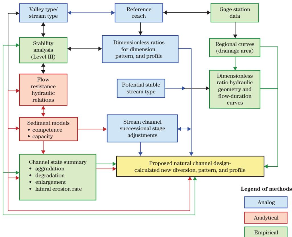
**Figure 11-17** Flowchart for determining sediment supply and stability consequences for river assessment
