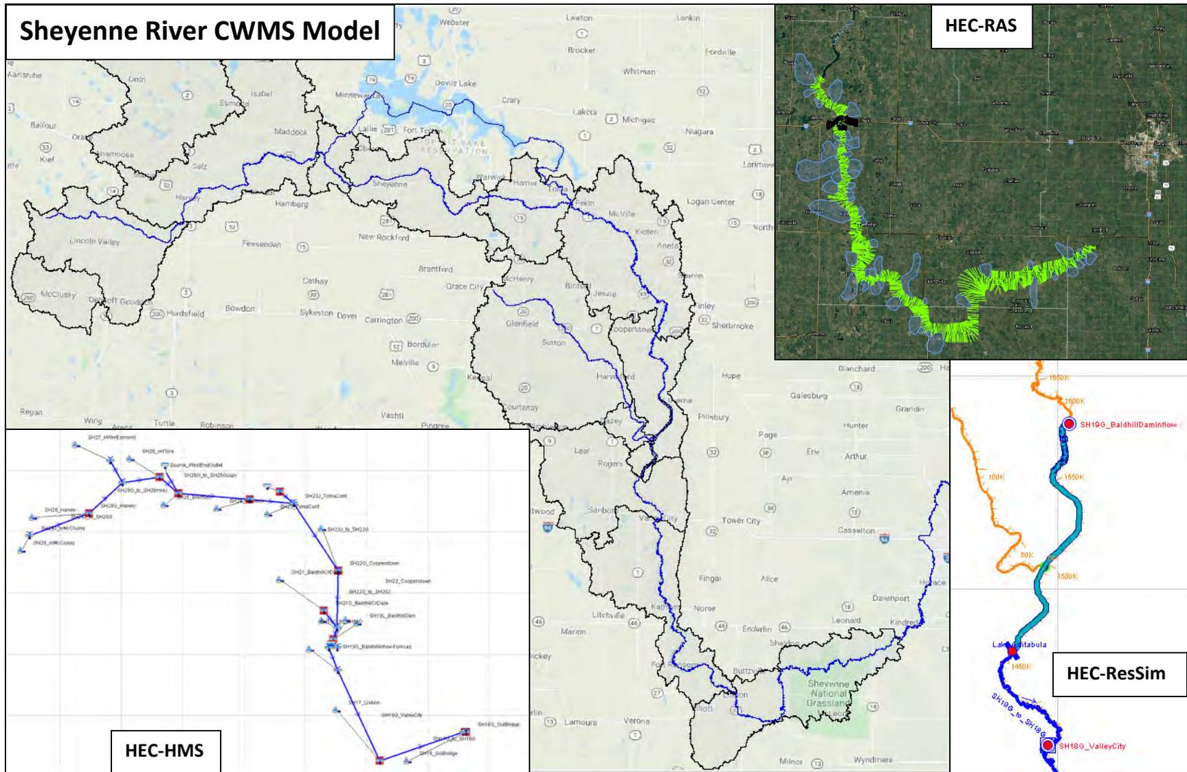
Figure 6. CWMS model interface and associated rainfall-runoff (HEC-HMS), reservoir operation (HEC-ResSim) and hydraulic models (HEC-RAS)
