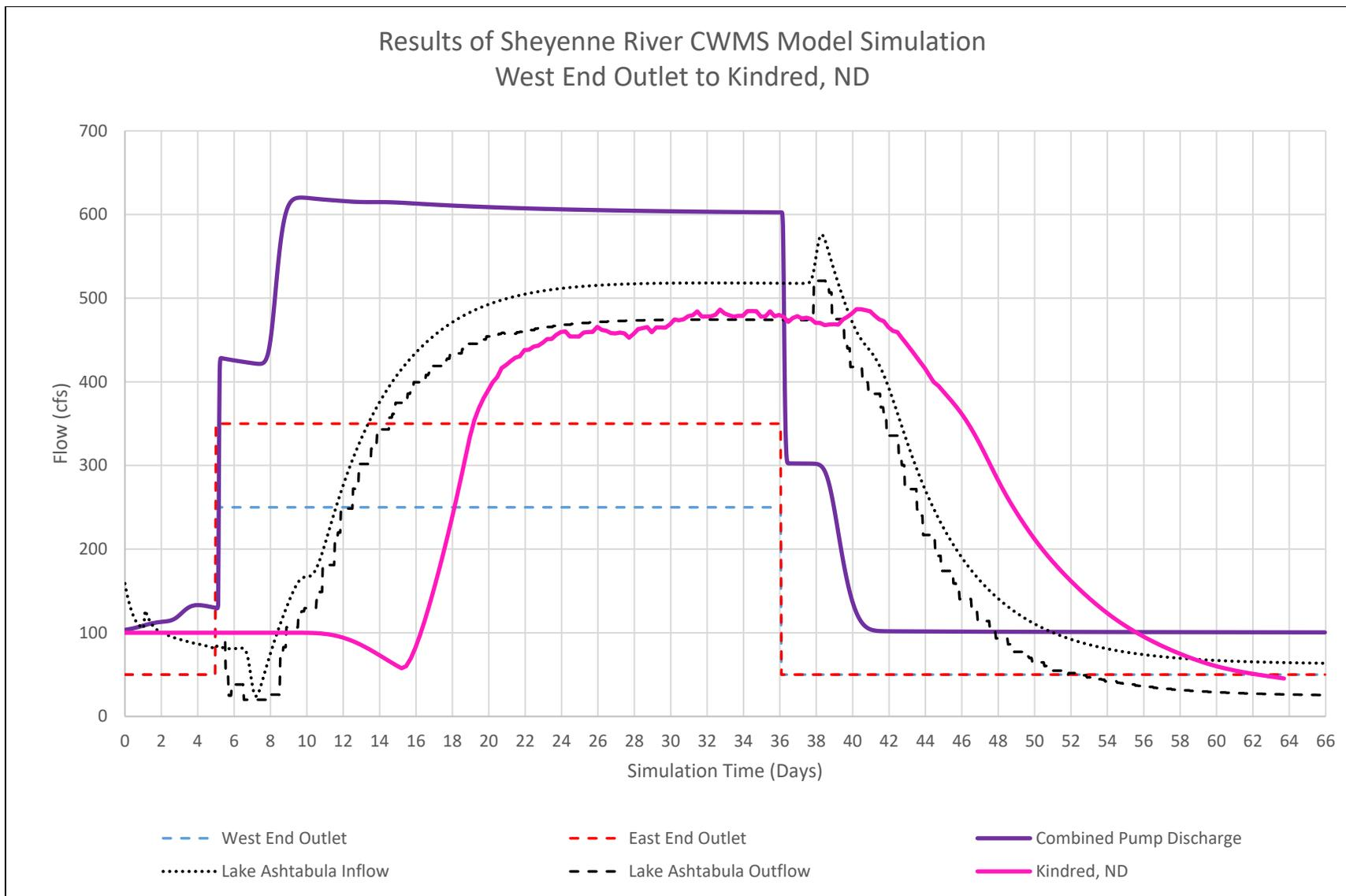
Figure 7. Results of CWMS routing model simulation
