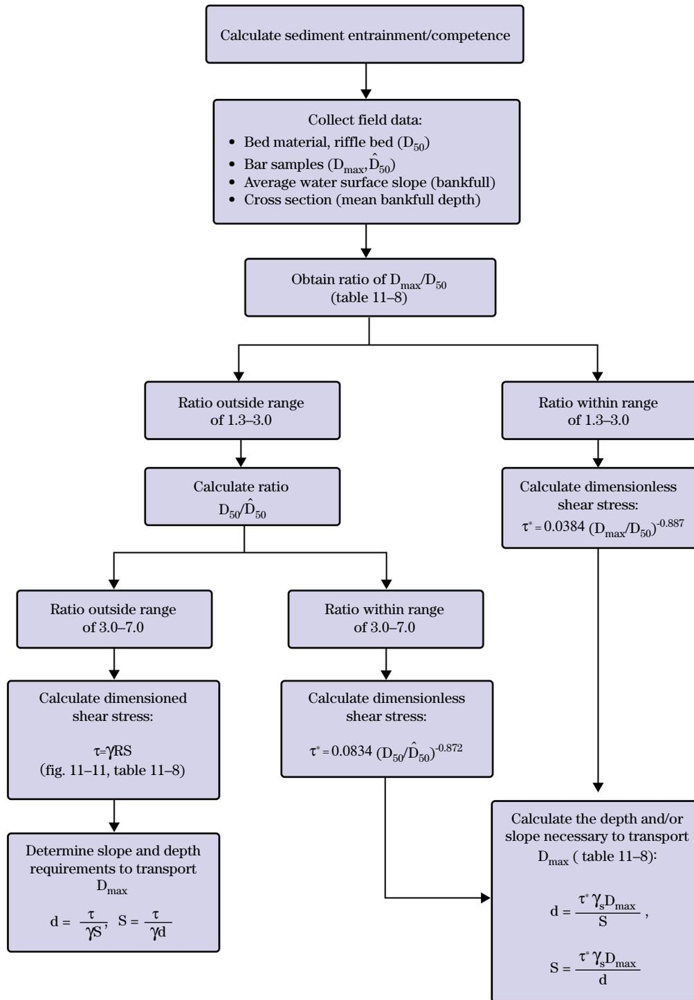
**Table 11-5** Field procedure for bar samples\***Bar sample field procedure**
