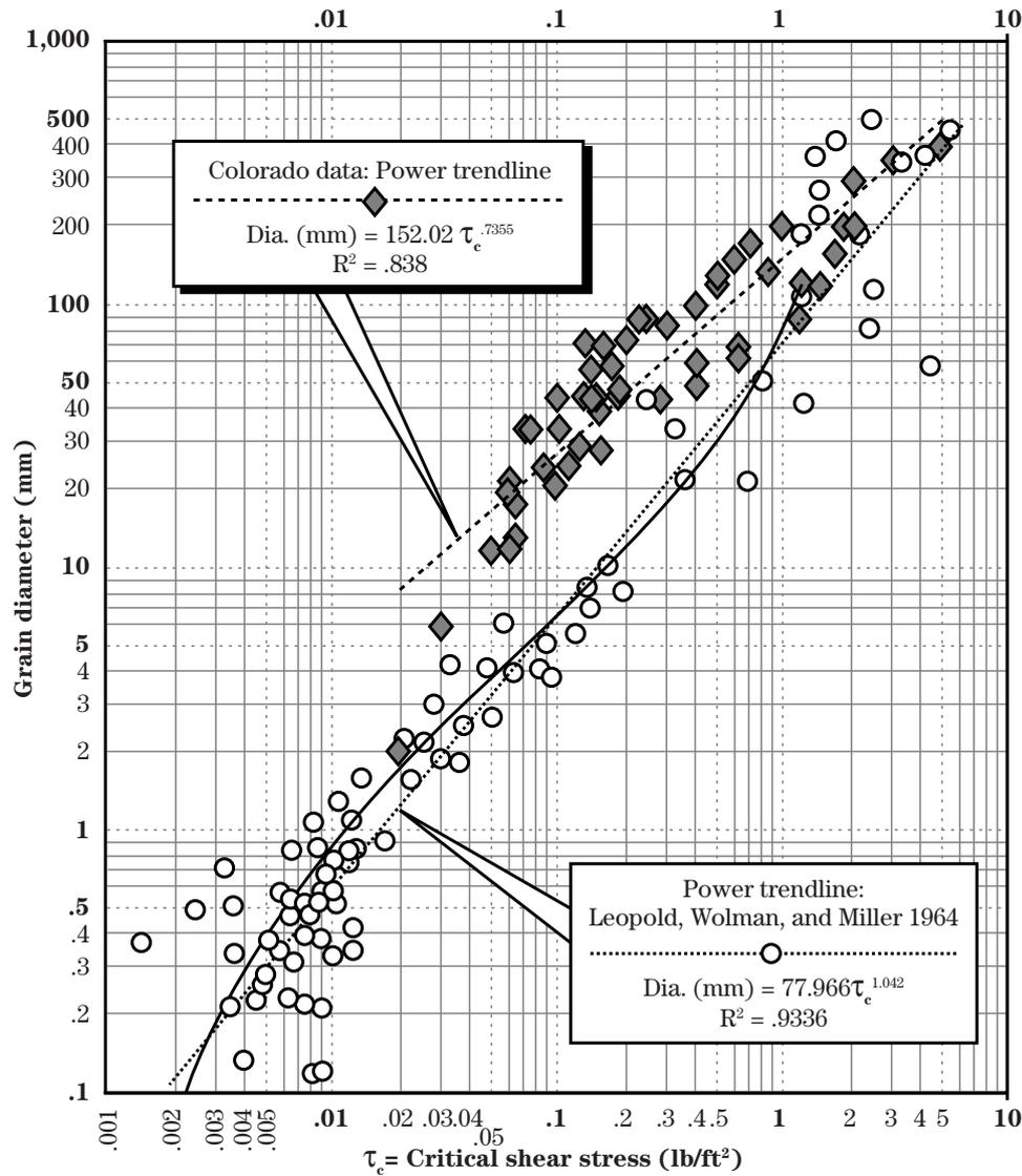
Laboratory and field data on critical shear stress required to initiate movement of grains (Leopold, Wolman, and Miller 1964). The solid line is the Shields curve of the *threshold of motion*; transposed from the  $\theta$  versus  $R_g$  form into the present form, in which critical shear is plotted as a function of grain diameter.
