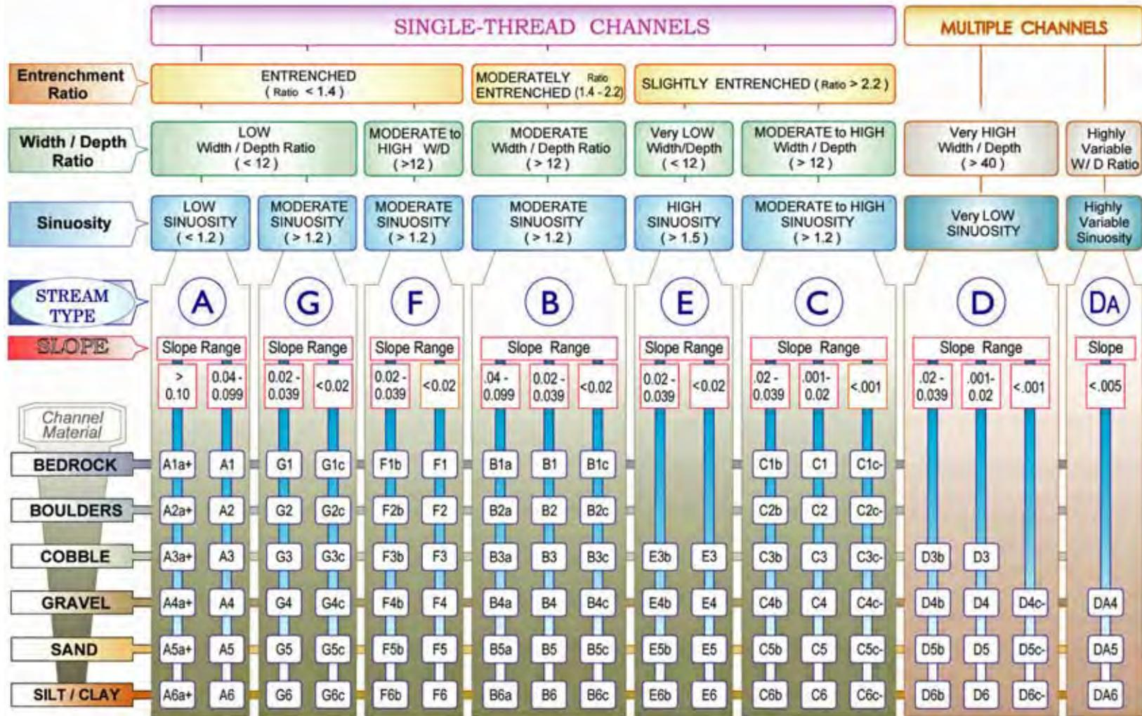
KEY to the **ROSGEN** CLASSIFICATION of NATURAL RIVERS. As a function of the "continuum of physical variables" within stream reaches, values of **Entrenchment** and **Sinuosity** ratios can vary by +/- 0.2 units; while values for **Width / Depth** ratios can vary by +/- 2.0 units.
