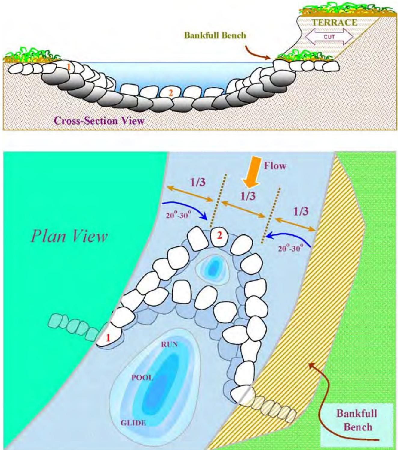
**Figure 11-42** Locations/positions of rocks and footers in relation to channel shape and depths
