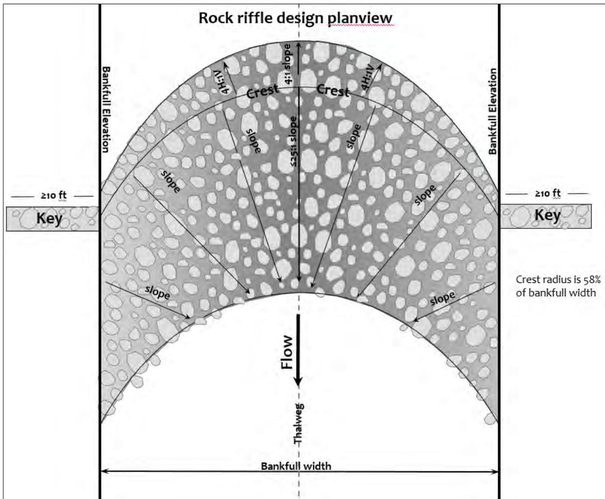
Figure 6-9: Generic Riffle Plan View Detail (Minnesota DNR)
