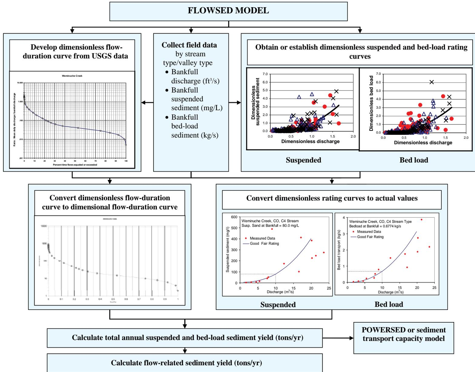
**Table 11-10** FLOWSED model procedure to calculate annual bed-load and suspended sediment yield**FLOWSED procedure**
