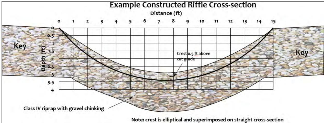
Figure 6-11: Generic Riffle Cross-Sectional View Detail (Minnesota DNR)
