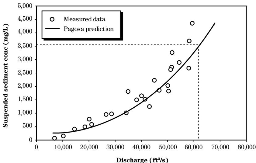
**Figure 11-13** Predicted vs. measured sediment data using reference dimensionless rating curve (data from Leopold and Emmett 1997; Ryan and Emmett 2002)
