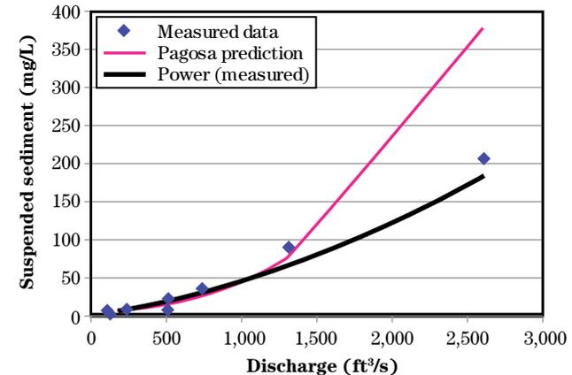
**Figure 11-14** Examples of predicted vs. measured suspended sediment data using dimensionless reference curve (data from Emmett 1975)—Continued
