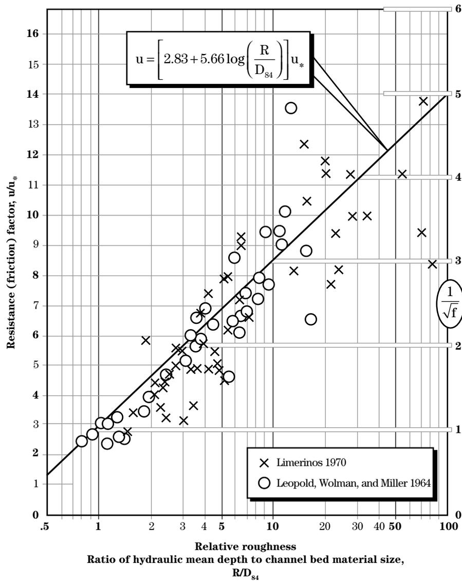
**Figure 11-7** Prediction of Manning's *n* roughness coefficient
