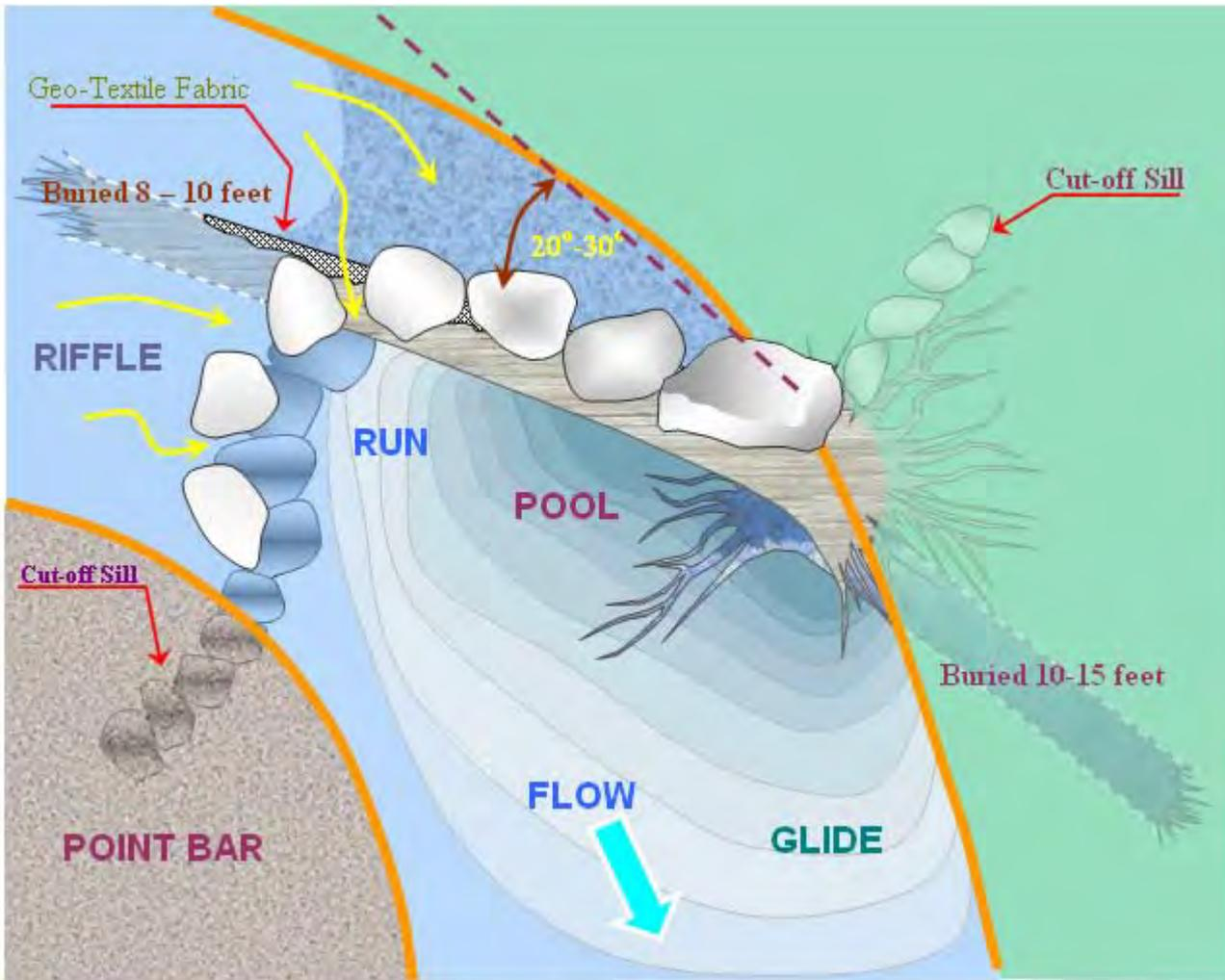
**Figure 11-37** Native boulder J-hook with cut-off sill, East Fork Piedra River, CO
