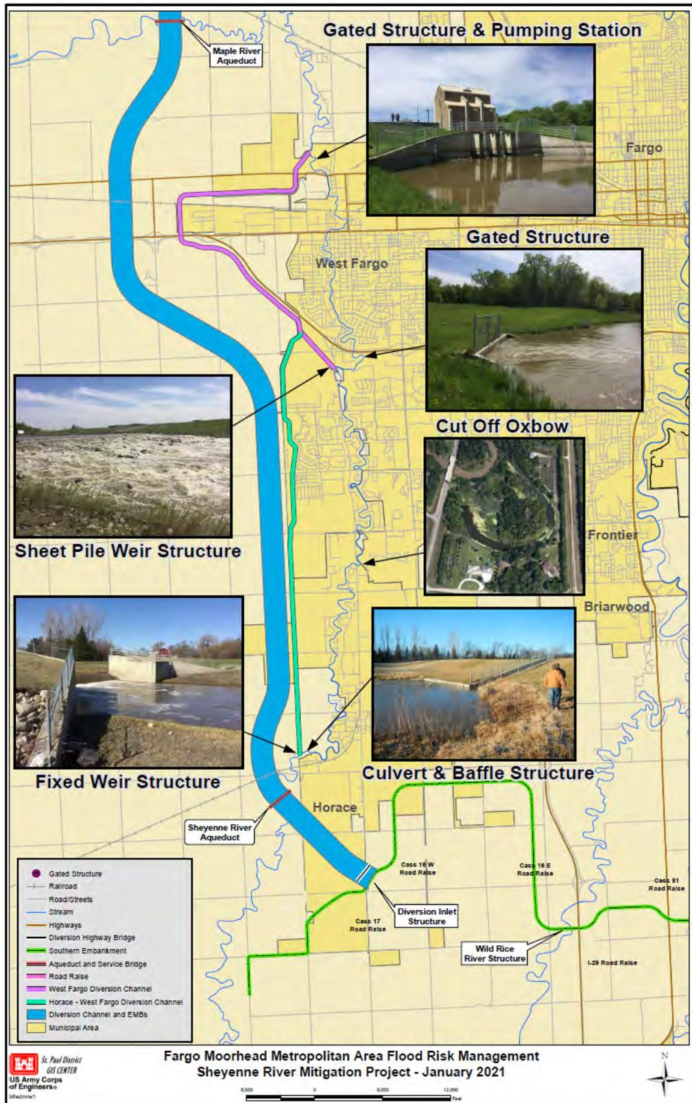
Figure 1. Overview of the Sheyenne River Flood Control Project (SRFCP) and associated features of the Sheyenne mitigation project.
