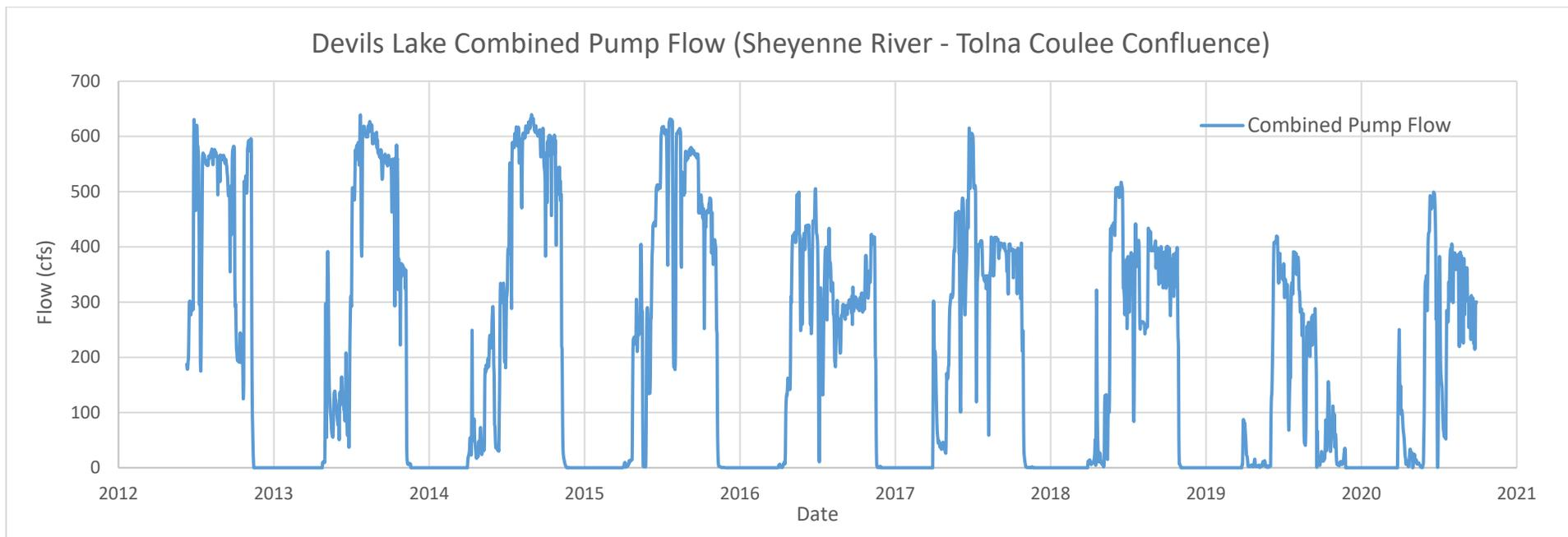
Figure 4. Discharge from the West End and East End outlets at Devils Lake, 2012-2020
