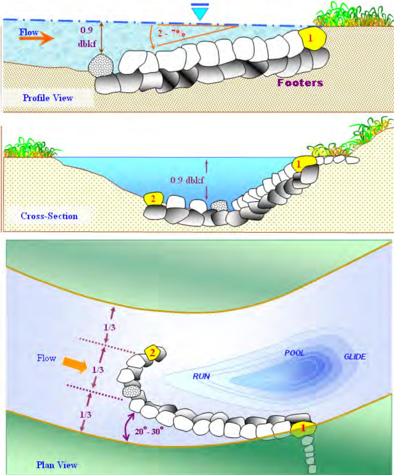
**Figure 11-35** Log vane/J-hook combo with rootwad structure
