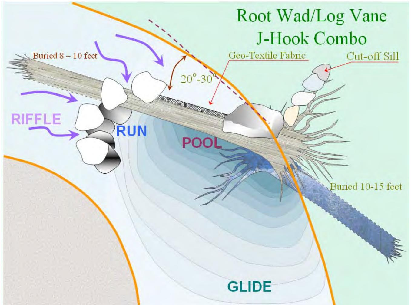
**Figure 11-36** Rock vane/J-hook combo with rootwad and log vane footer
