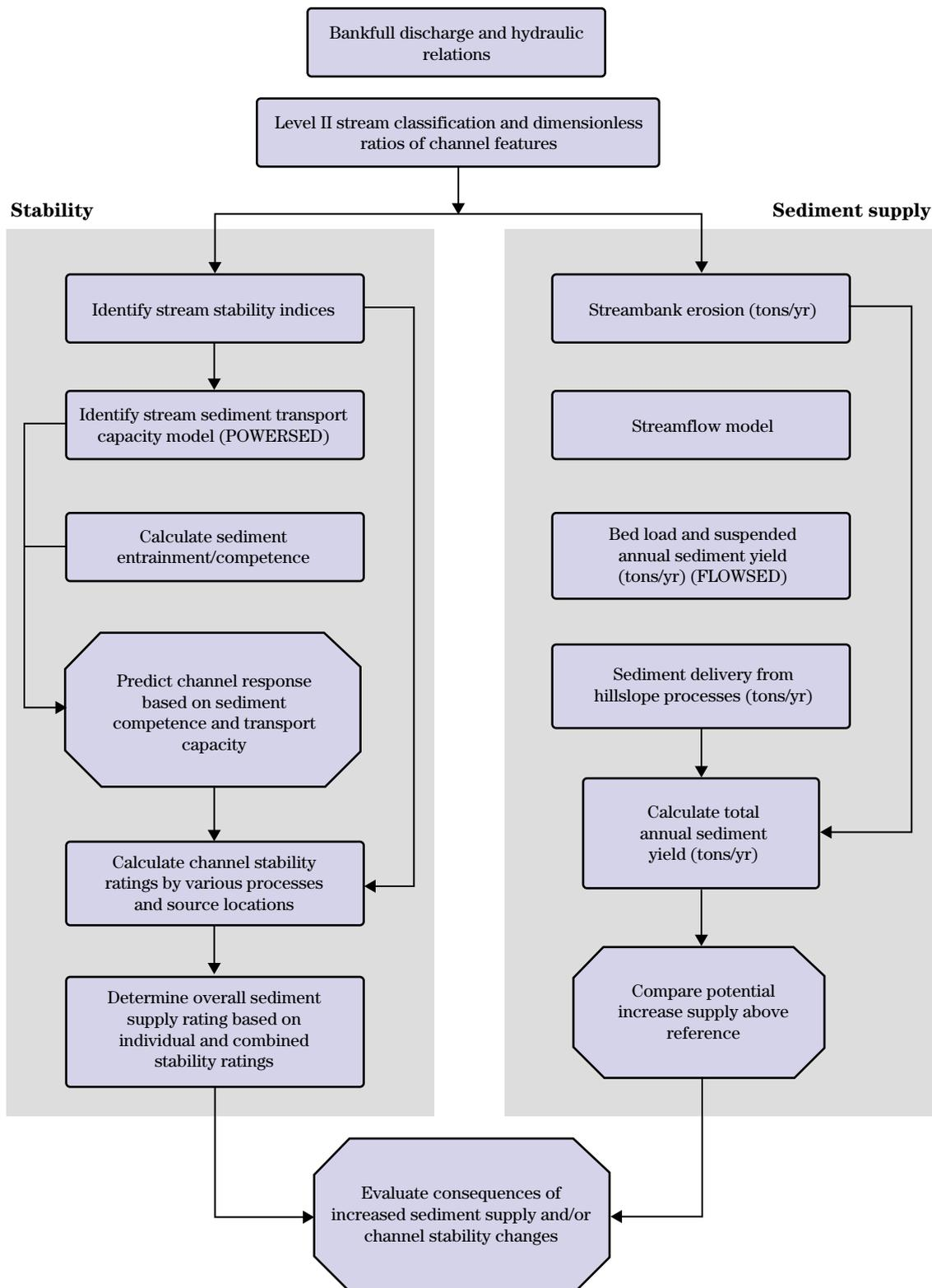
The procedural sequence utilized in the Rosgen geomorphic channel design methodology is shown in the following operational steps:
