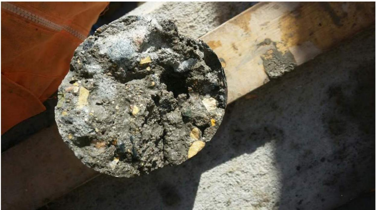
Figure 8: Void in Core #1
