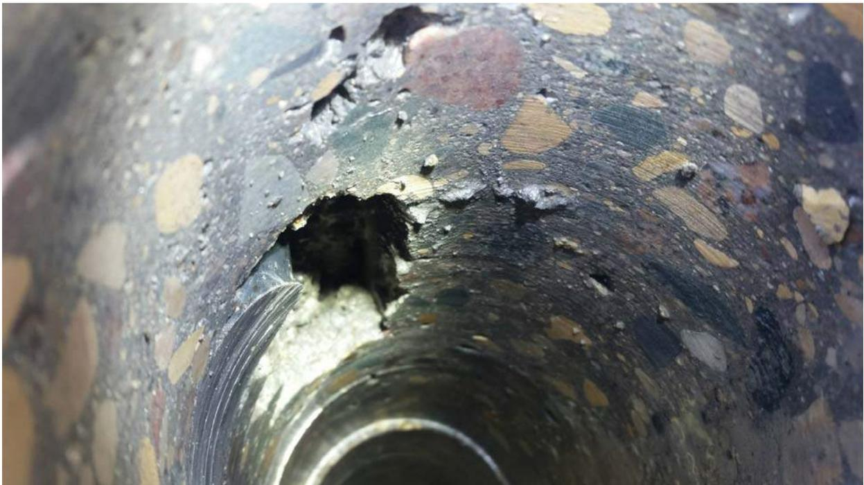
Figure 10: Void in Core Hole #1
