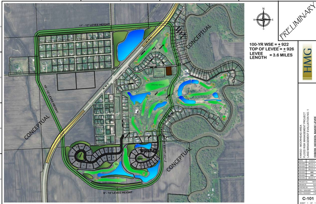
Figure 4. Oxbow, Hickson, and Bakke Levee Alignment.
