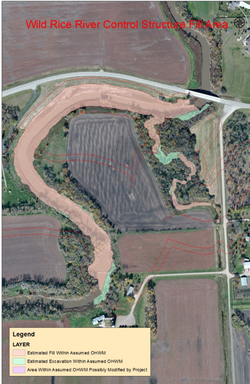
Figure 3. Wild Rice River Control Structure Fill Area.
